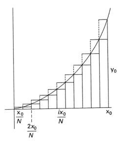
Divide the interval from x=0 to x=x<sub>0</sub> into N subintervals under the curve  $y=px^k$  produces the expression for the sum of the areas of the rectangles
