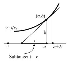
Fermat gives the formula ("the adequality") needed to find the tangent to a curve y=f(x) at (a,b) as
