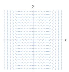
14. Because f depends only on y (the equation is autonomous), the slope field is constant along horizontal lines in the ty-plane. The roots of f correspond to equilibrium solutions. If f(y) > 0, the corresponding lines in the slope field have positive slope. If f(y) < 0, the corresponding lines in the slope field have negative slope.
